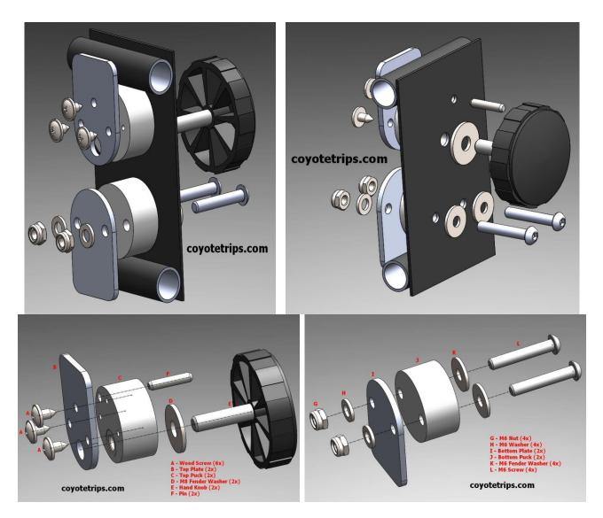
12. Mount the pucks and plates as shown in the images above. The nut M8 inserted into the upper puck needs to face the aluminum plate, away from the pannier. Make sure not to over-tighten the sheet metal screws.
